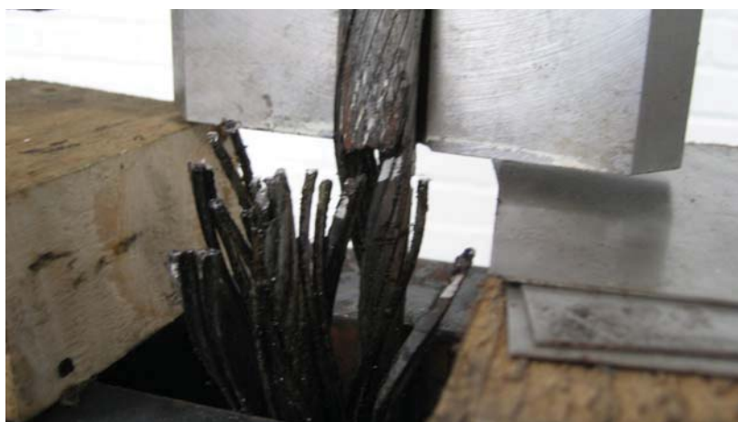
Figure 10: Clamp lower exit point at which the main failure occurred. Note the Z wires which were at the 'sides' of the clamp groove have not failed. Note also the fretting rouge at the position of the rope just inside the clamp.
