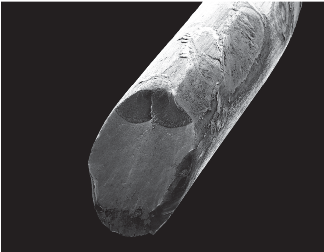
Figure 14: An internal round wire. Two adjacent fatigue cracks have started at points of contact with neighbouring wires. The wire finally failed in shear. (approximate magnification \times 15 ).
