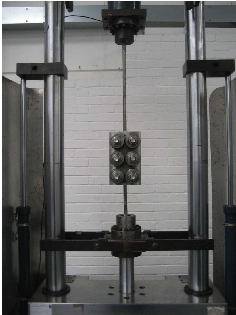
Figure 6: General view of rope safety clamp installed on a FLC rope tensile fatigue sample.
