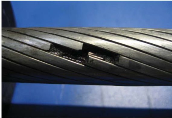
(a) Two wire breaks at 25 mm
